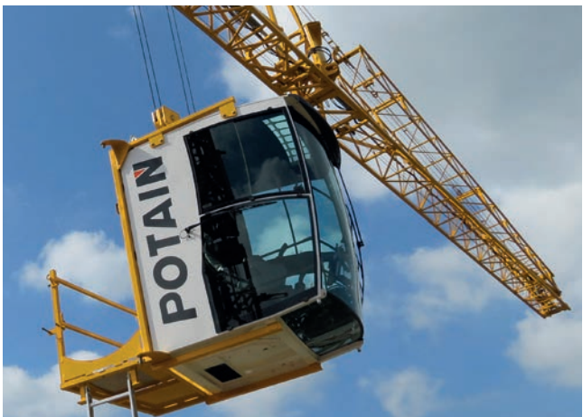
Fitting the cab By the crane itself (without additional equipment)
