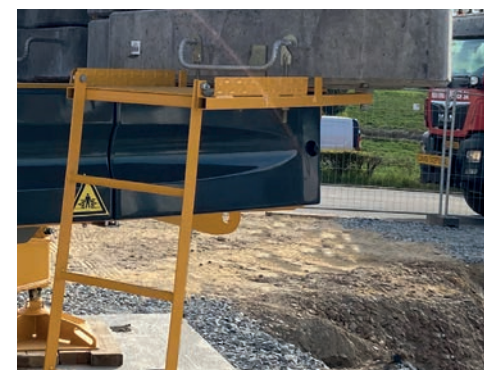
Access platform to the ballast slabs (standard)
