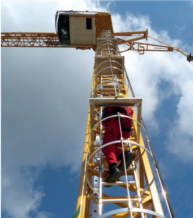
Cab access (ladders + rungs) entirely positioned outside the mast and in compliance with the latest regulations.
